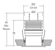
IP54 rated Version supplied with an extra gasket between the bezel and mounting surface
